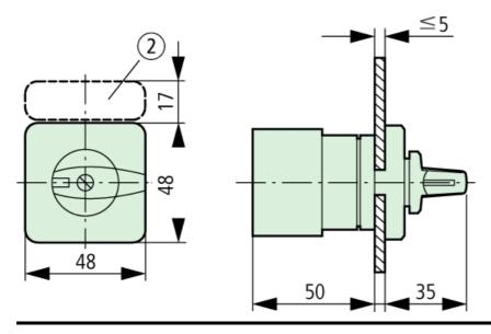
not included Depth of one contact unit: 9.5 mm
