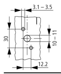
Diameter of drilled hole Door
